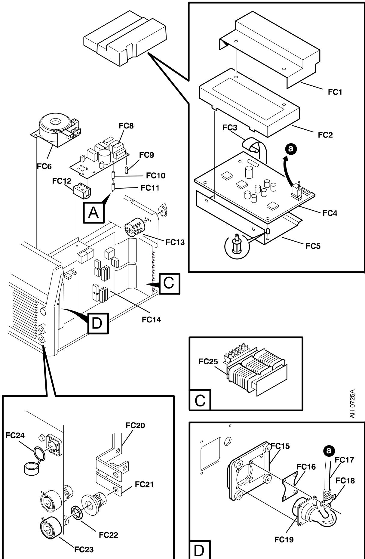
***Mig L3000i, Mig C3000i,******AristoMig 300, ESABMig 300i, AristoMig C300, ESABMig C300i*****C = component designation in the circuit diagram**
